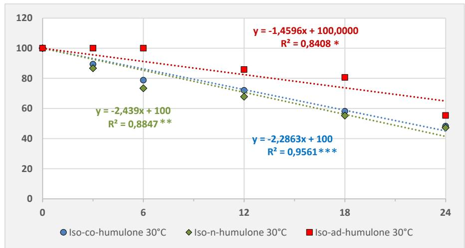
Fig. 5 The change in the homologues of the iso- $\alpha$ -acids (late-hopped beers) during ageing, shown with a regression line over a period of 24 months
